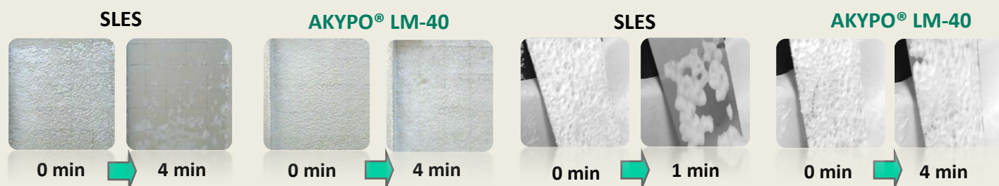
Formula based on AKYPO ® LM-40 remains on the surface for more than 10 minutes
